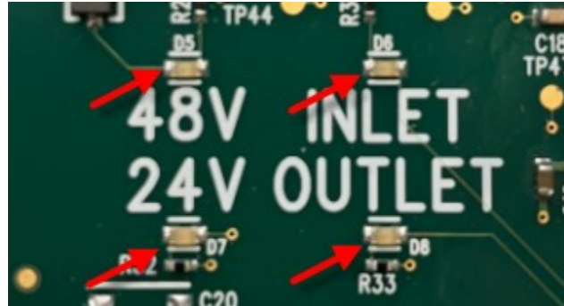
Figure 18. 48 V and 24 V LEDs
