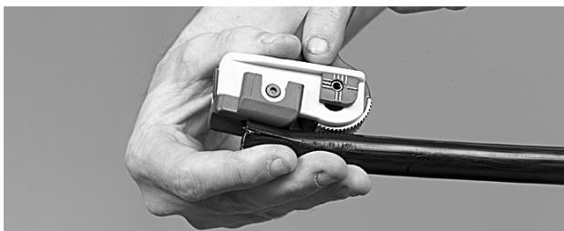
2 The eccentric unit has been adjusted correctly, if the plate of the cutter is parallel with the cable while the blade is inserted under the cable sheath.
