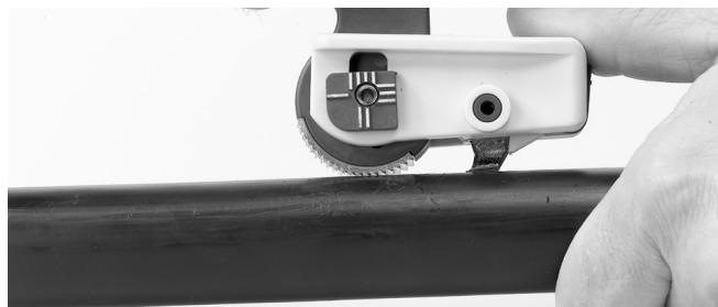
4 For longitudinal cutting of uncut cables use eccentric position IIII. The cable sheath is cut by holding the blade against the cable sheath and pressing down the hand lever. After the blade has penetrated the cable sheath, set the eccentric unit to the appropriate position and make the desired longitudinal cut.
