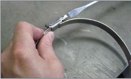
Step 1 - Unscrew the clamp
