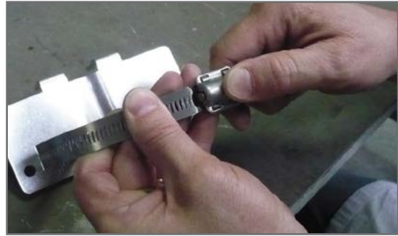
Step 4 - Insert the free terminal of the clamp into lock
