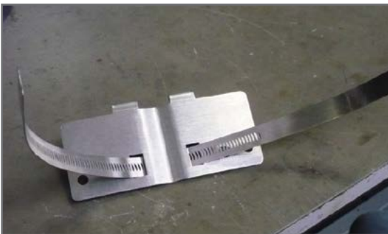
Step 3 - Insert clamp into bracket
