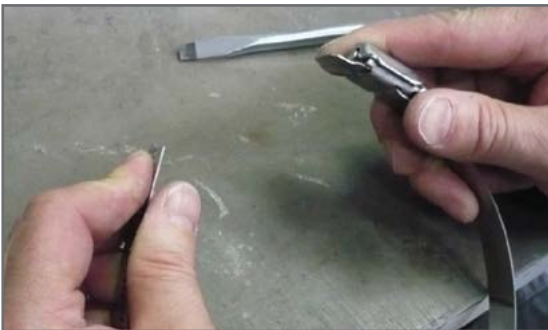
Step 2 - Open the clamp
