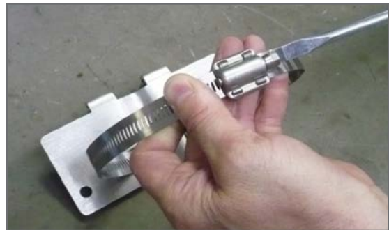
Step 5 - Tighten the screw along the band up to the required torque (recommended 7.5 to 10Nm max) by means of a screwdriver
