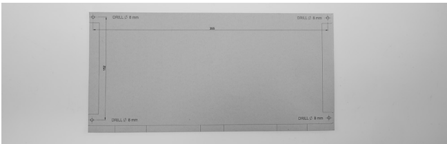
1.2 Use the template to mark the drill holes.
