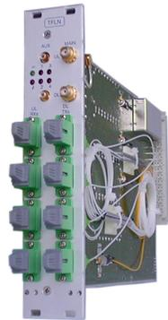
ION®-B Series Master Optical Transceiver, 380–960 MHz
